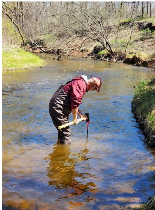
Figure 6 Volunteer installing rebar with thermistor into stream (Photo credit: Laura DeGolier)
