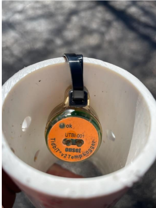
Figure 3 Tidbit V2 thermistor in PVC housing
