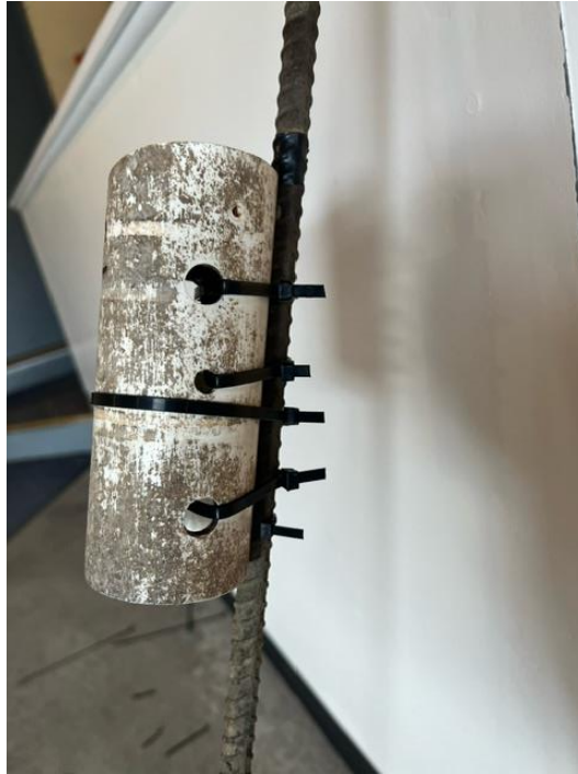
Figure 5 PVC housing with thermistor inside zip tied to rebar (Photo credit: Gary Hermann)
