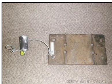
Connect to PVC tube with zip ties and attach to railroad plate or rebar. Wedge plate or pound rebar into streambed.
