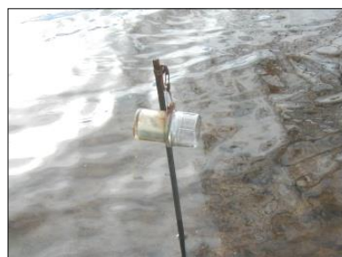
Connect to PVC tube with zip ties and attach to railroad plate or rebar. Wedge plate or pound rebar into streambed.
